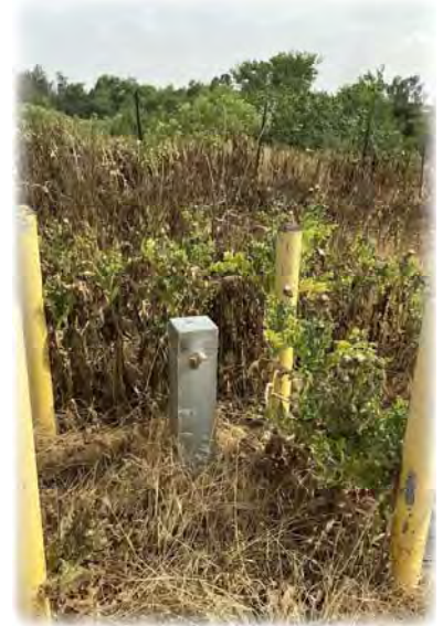
Prado Basin Monitoring Well
